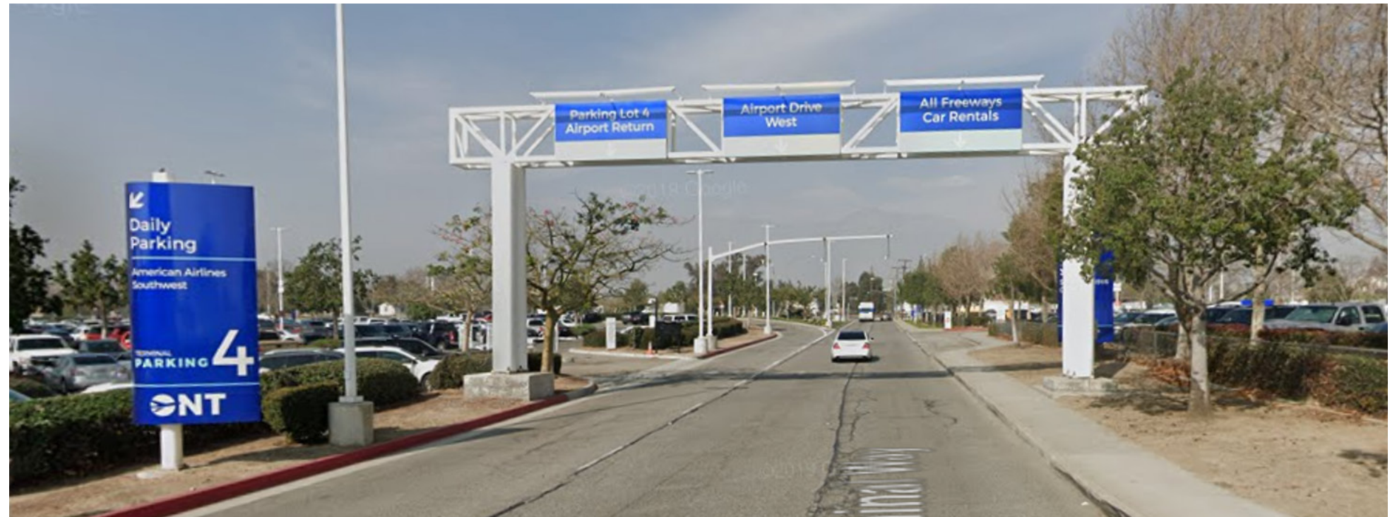
The use of branding colors, in the case of this overhead roadway sign, has resulted in the directional areas being hard to read.
